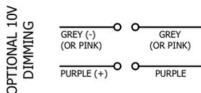
**NOTE: DIMMING LEADS (0-10V): PURPLE (DIM +) AND GRAY (DIM -) LEADS TO BE INDIVIDUALLY CAPPED OFF IF UNUSED; NOT TO BE CONNECTED TOGETHER.**
