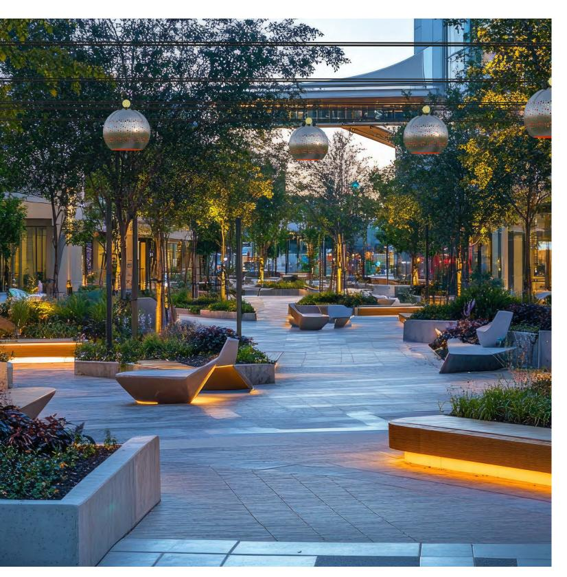
The TWS12 is a heavy-duty aluminum catenary fixture, designed to provide both durability and striking illumination for urban environments, public spaces, and hospitality settings. Built to withstand the elements, the LED module and driver are IP66-rated, ensuring long-lasting performance in demanding outdoor conditions.
