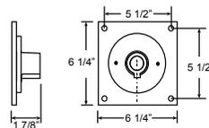
**CAST BACK PLATE MOUNTING DETAIL**
