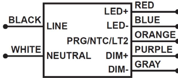
**Note:** Maximum suggested remote mounting distance is 16 feet. For additional information on further distances and EMI compliance reference application note LED126.
