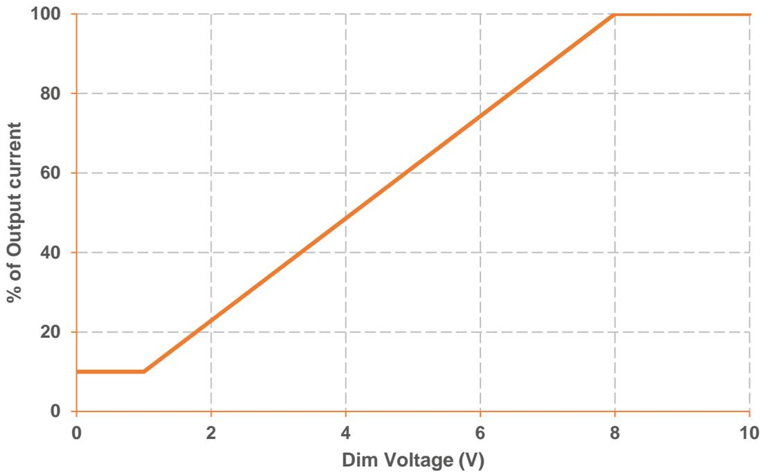
\*The absolute minimum current the driver can deliver is 50mA
