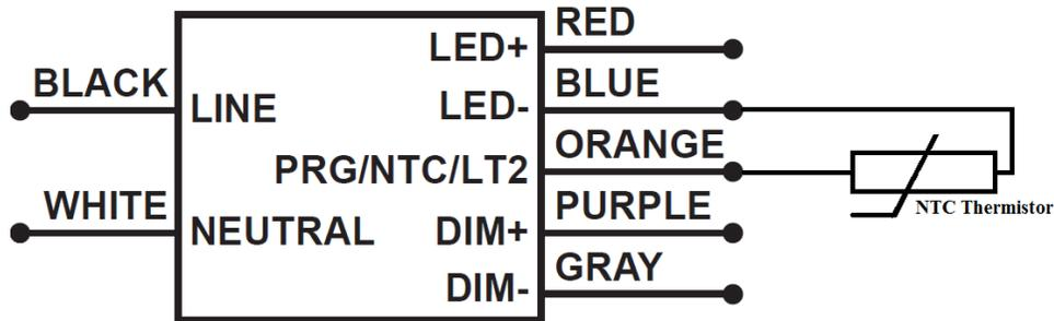
In the end application, care must be taken to place the NTC thermistor close to the hottest spot on the LED module. If LED thermal protection is not required the NTC port on the LED power supply connector can be left open.
