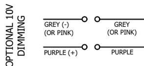
**NOTE: DIMMING LEADS (0-10V): PURPLE (DIM +) AND GRAY (DIM -) LEADS TO BE INDIVIDUALLY CAPPED OFF IF UNUSED; NOT TO BE CONNECTED TOGETHER.**
