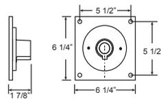
**CAST BACK PLATE MOUNTING DETAIL**
