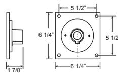
**CAST BACK PLATE MOUNTING DETAIL**
